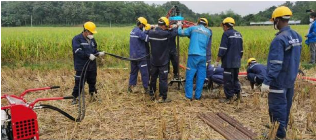
Figure 6: Seismic drilling in a 2D seismic survey over exploration blocks 15 and 22 by BAPEx
