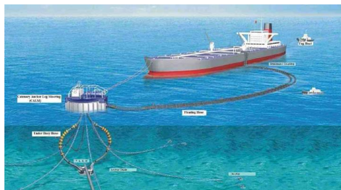
Figure 8: Single Point Mooring (SPM) with Double Pipeline
