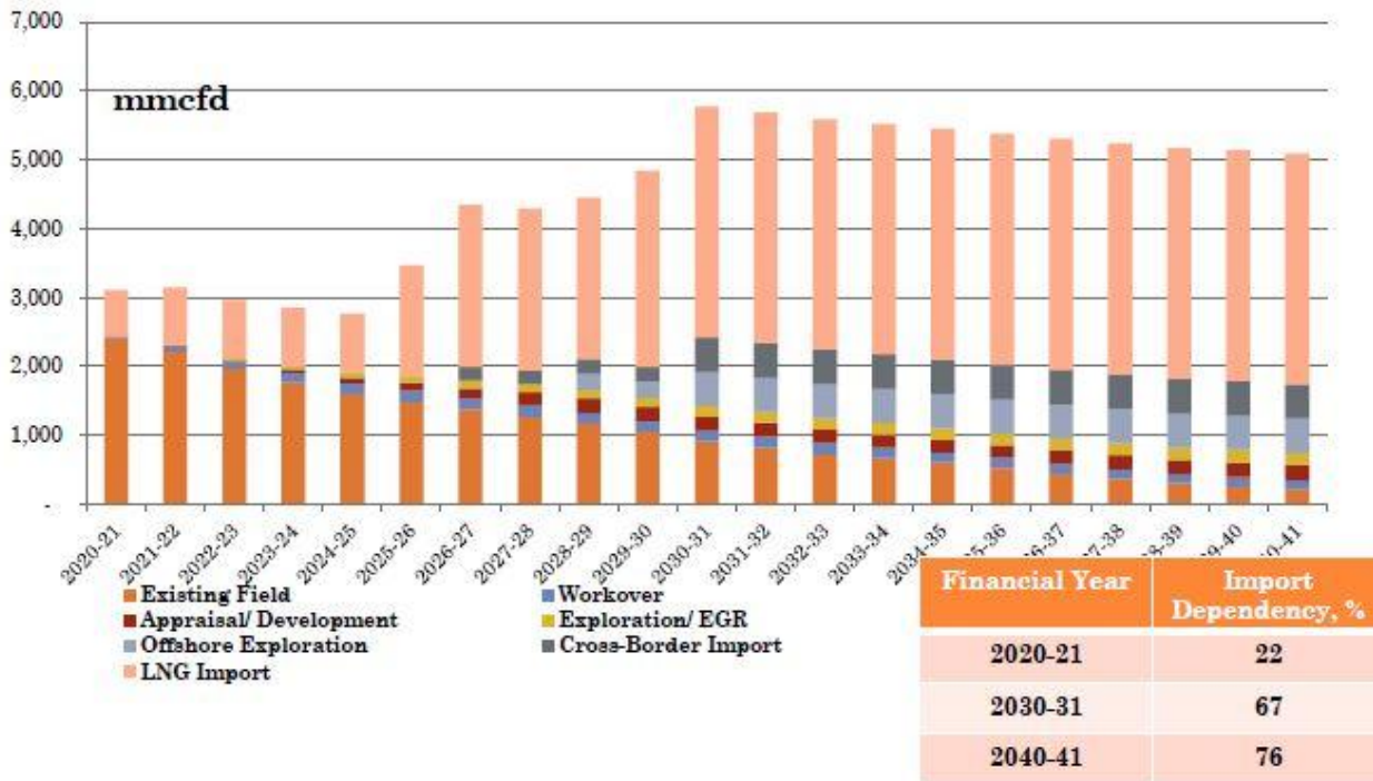
Figure 26: Gas supply projection
