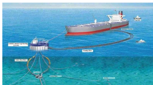
Figure 9: Single Point Mooring (SPM) with Double Pipeline
