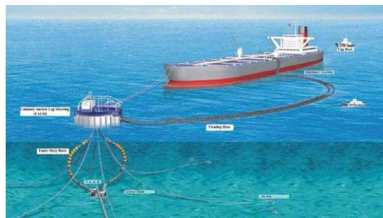
Figure 12: Single Point Mooring (SPM) with Double Pipeline
